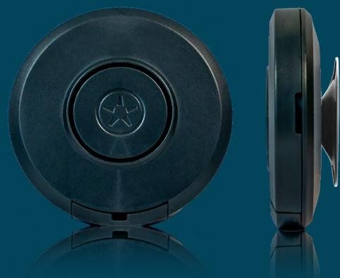
The Compact Button is a long-range vehicle identification tag. This tag is based on semi-active RFID technology. It operates on a frequency with very little interference or environmental noise. In addition, the tag is battery powered to give a strong response signal, which makes it the most accurate and reliable identification system. The read-range is up to 15 meters\* (50 feet) in combination with the TRANSIT Ultimate reader.
